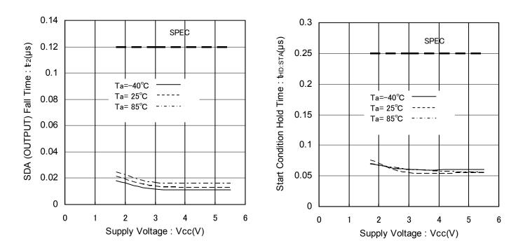
Figure 16. SDA (OUTPUT) Fall Time vs Supply Voltage
