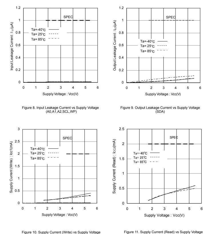
Figure 11. Supply Current (Read) vs Supply Voltage  $(f_{\text{SCL}}=1MHz)$
