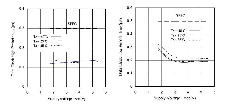
Figure 14. Data Clock High Period vs Supply Voltage
