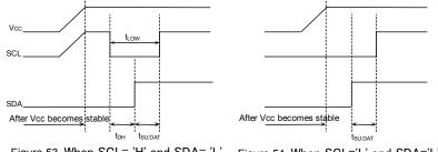
Figure 53. When SCL= 'H' and SDA= 'L' Figure 54. When SCL='L' and SDA='L'
