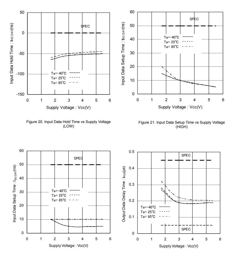
Figure 22. Input Data Setup Time vs Supply Voltage Figure 23. Output Data Delay Time vs Supply Voltage
