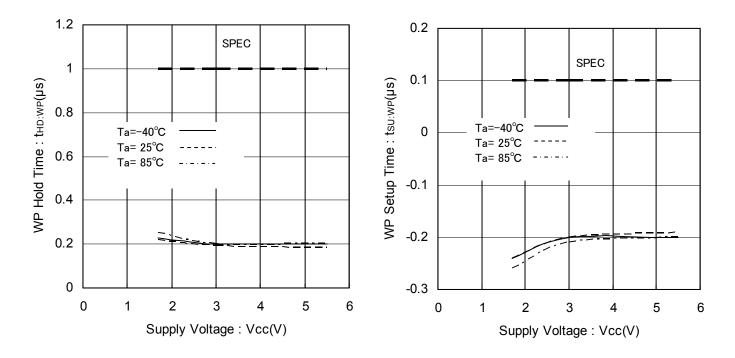
Figure 32. WP Hold Time vs Supply Voltage
