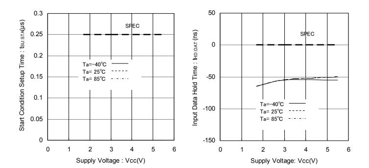
Figure 18. Start Condition Setup Time vs Supply Voltage
