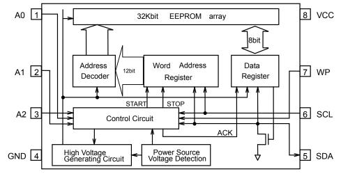
Figure 3. Block Diagram
