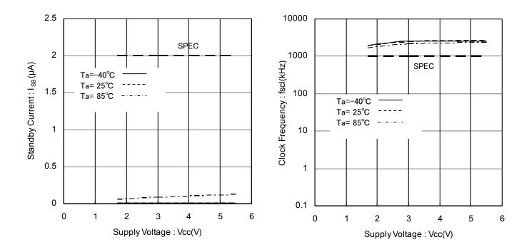
Figure 12. Standby Current vs Supply Voltage
